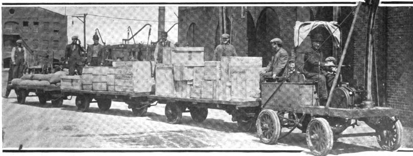
Battery crane truck for handling light freight at Bush Terminal. Giant warehouse in background
